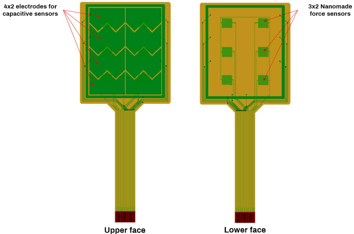
This sensor is designed on a double side FPC. There are 8 electrodes for capacitive sensor on the upper layer and 6 force sensors on the bottom layer. This configuration allows multipoint touch and force sensing.
