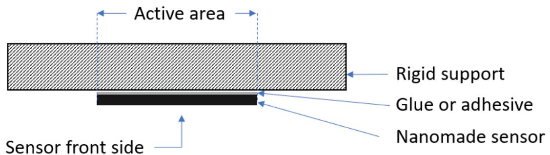
The higher the deformation transmitted to the sensor, the higher the variations of the sensor signal output. Thus, it is recommended to use rigid curing glue, as for example Cyanoacrylate. However, for an easier integration, it is also possible to use double sided tape adhesive, as for example 3M VHB F9460PC.
