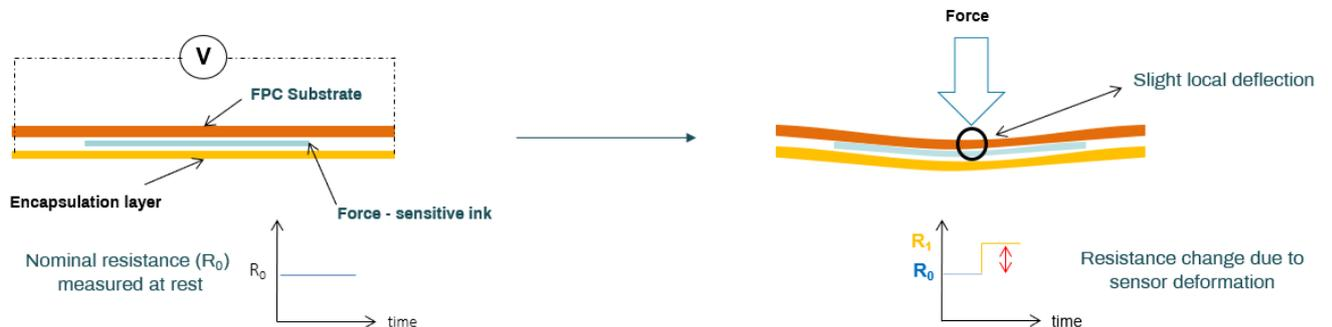
When a strain is applied, a measurable change in the electrical resistance of the sensor is detected. The higher the pressure applied, the higher the resistance change.
