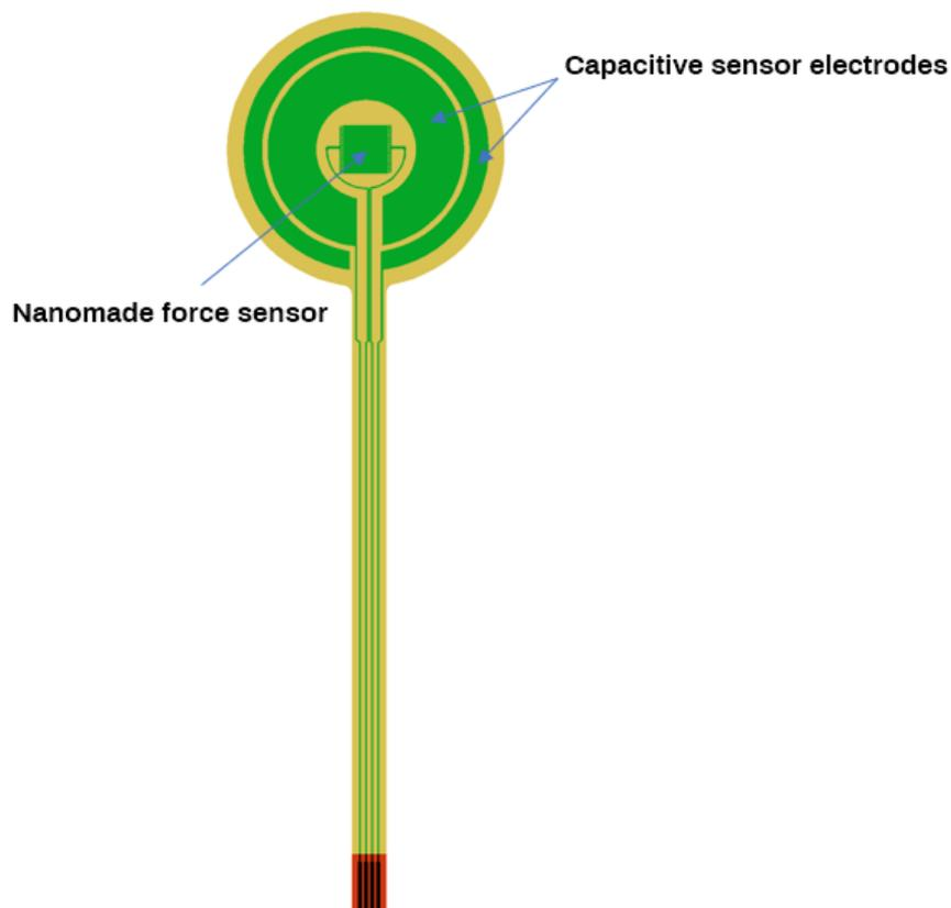
This sensor is composed of only one copper layer on polyimide substrate. Both capacitive and force sensors electrodes are designed on this unique layer.
